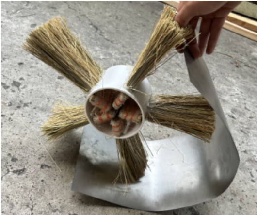
Fig. 4. Second prototype of broom mechanism to pick up baseballs in a wheel well
