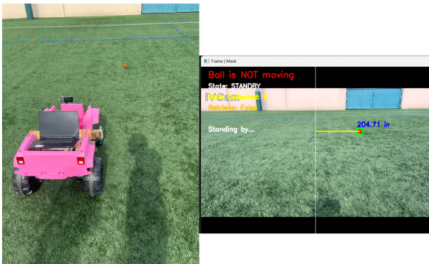
Fig. 10. Final prototype of rover displaying end goal of autonomously picking up baseballs
